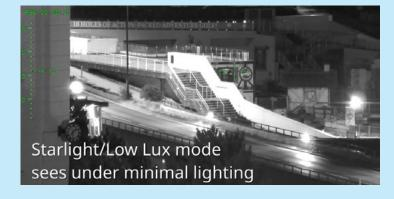
IR and Low light modes, In low light conditions the EO camera goes into 'starlight' mode – it can see much better than the human eye at night, combine this with Infra-Red mode and the scene is clear, objects and targets may easily be seen at long range.
